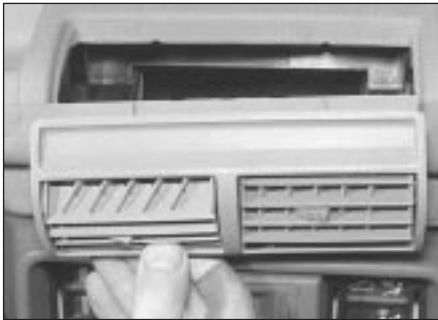
26.4 Removing the central air vents
