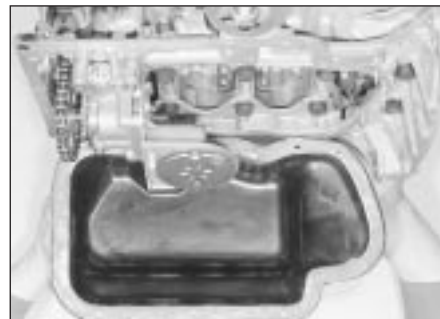
12.5 Slacken and remove the sump nuts and bolts, then remove the sump
