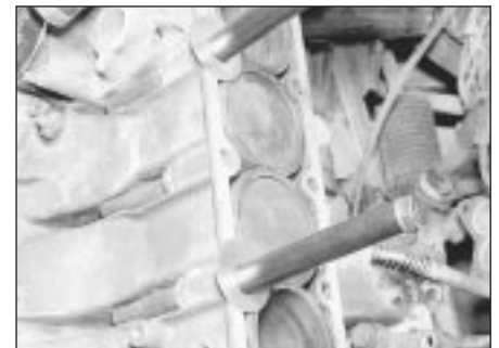
7.32 Using washers, tubing and the cylinder head bolts to clamp the liners in position
