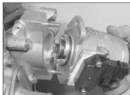
4.18 . . . then remove the distributor
