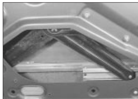
12.2b The window regulator lifting arms and window glass channel
