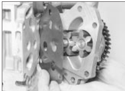
4.10b Removing the oil pump and spacer plate
