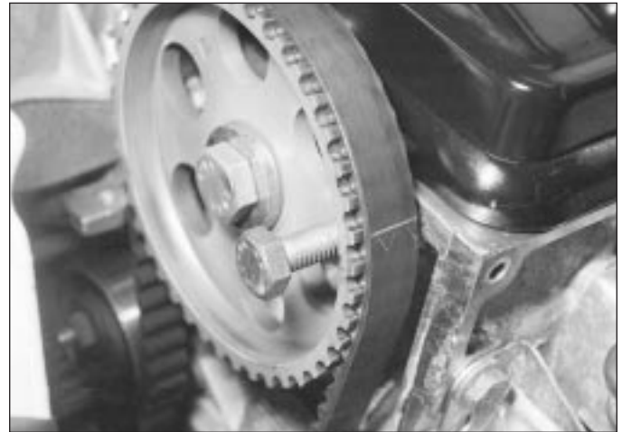
3.5 . . . then insert a 10 mm bolt through the camshaft sprocket timing hole, and locate it in the cylinder head
