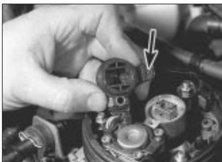
11.13 Intake air temperature sensor (arrowed)
