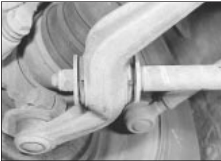
6.2 Anti-roll bar attachment to lower suspension arm on non-GTI models
