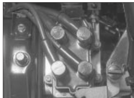
6.5 HT lead connections on the static distributorless ignition module
