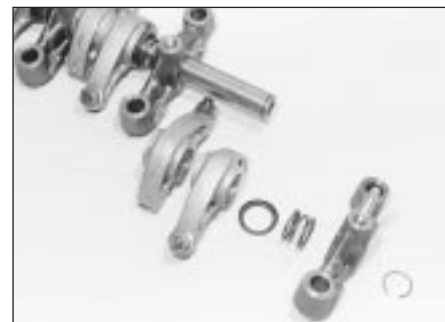
10.4 Remove the circlip, and slide the components off the end of the rocker shaft
