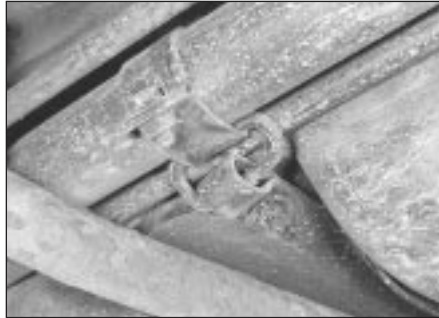
11.6 Rear suspension cross-tube front clamp and seat belt anchorage
