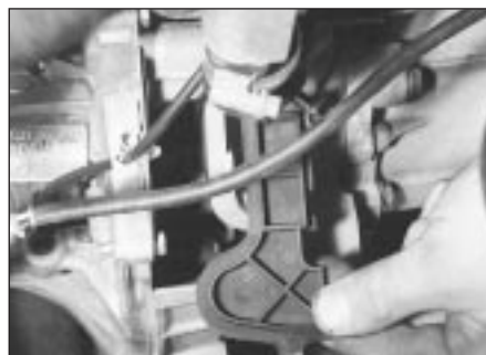
8.25a On TU series engines, remove the plug from the transmission housing . . .
