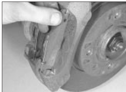
4.5 Removing the outer pad (DBA Bendix caliper)
