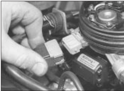
11.23a Disconnecting the wiring plug from the fuel injector . . .
