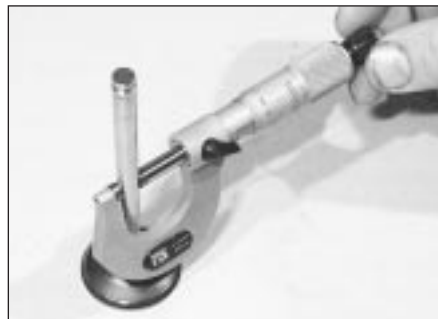
6.18 Measuring the valve stem diameter
