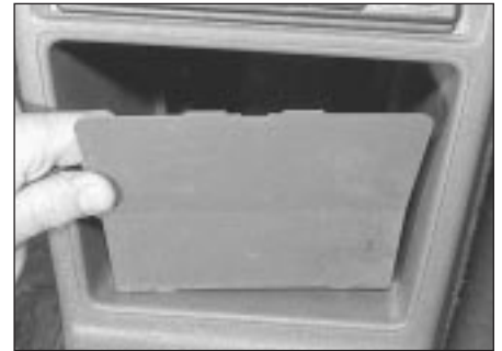
26.6 Removing the rear of the ashtray tray
