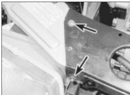
5.2 Undo the bolts (arrowed) on each side and lift off the front crossmember
