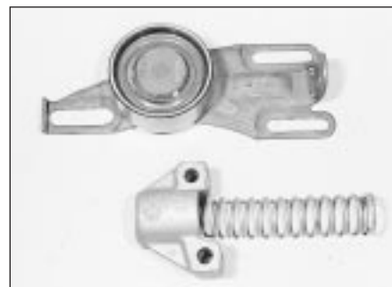
5.12 Spring loaded timing belt tensioner components
