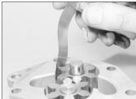
5.6 Checking oil pump gear to body clearance
