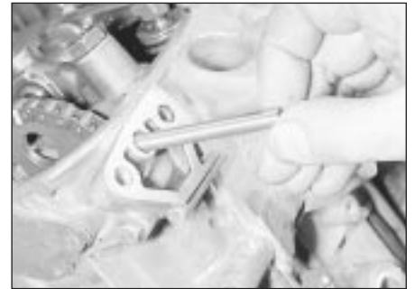
7.21 Removing the fuel pump plunger
