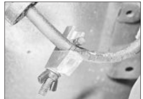
10.5 To minimise fluid loss, fit a brake hose clamp to the flexible hose
