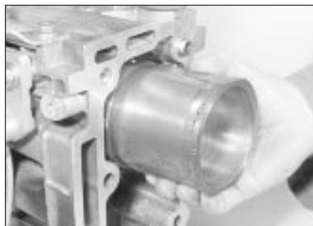
9.36 Fitting a liner to the cylinder block
