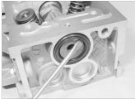
10.9a . . . prise out the oil seal . . .
