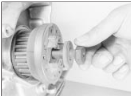
8.11a Remove the crankshaft sprocket bolt . . .
