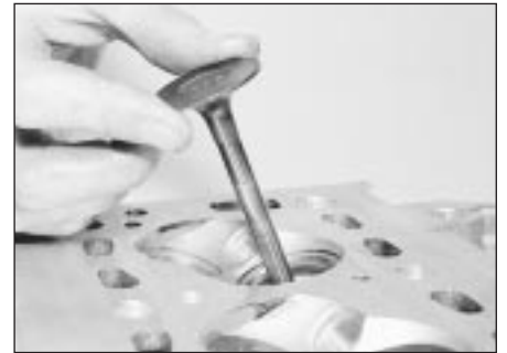
6.6 Withdraw the valve through the combustion chamber
