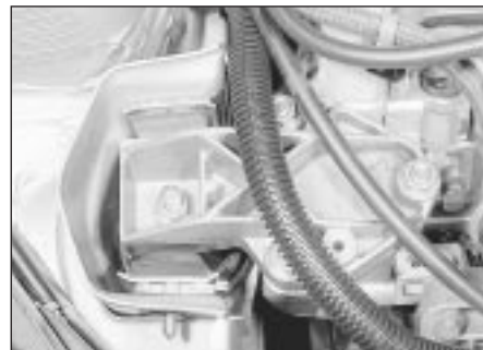
8.6 Right-hand engine mounting and cylinder head bracket
