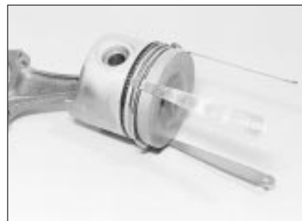
7.18 Using old feeler blades to assist removal of the piston rings
