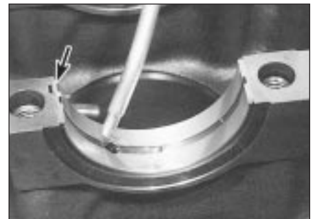
13.71 Ensure each bearing shell tab (arrowed) is correctly located and apply clean oil
