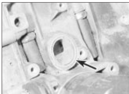
8.3c . . . and recover the O-ring - arrowed (XV, XW and XY series engines)
