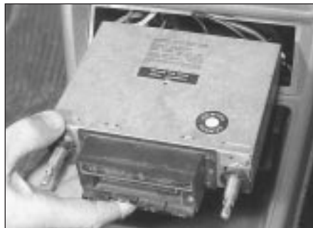
22.3 Removing the radio on early models
