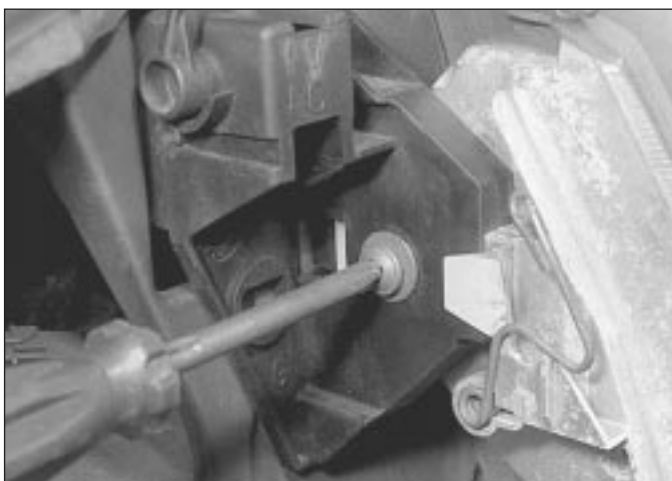
11.3a Remove the headlight adjustment assembly screw . . .
