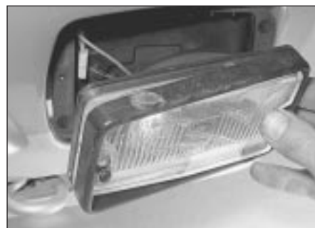
8.15 On GTI models, remove the driving light lens surround, lens and reflector ...
