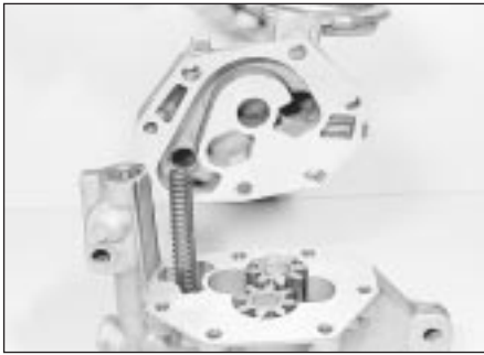
10.5a Lift off the pump strainer cover . . .
