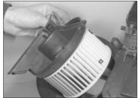
9.7 Removing the heater blower motor
