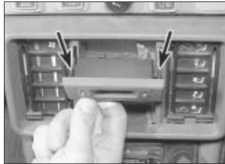
26.5 Digital clock and retaining barbs (arrowed)
