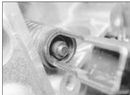
6.4a Compress the valve spring with a compressor and remove the split collets . . .
