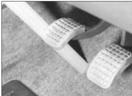
10.2 To check the clutch pedal stroke, measure the clutch pedal travel as described in the text
