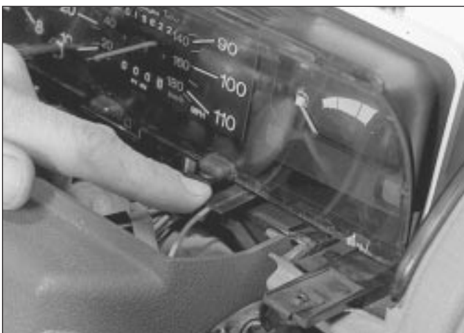
5.6a Instrument panel spring support
