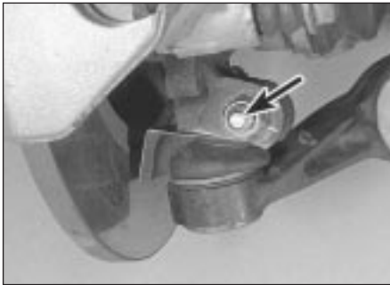
2.4a Unscrew the lower balljoint clamp bolt . . .
