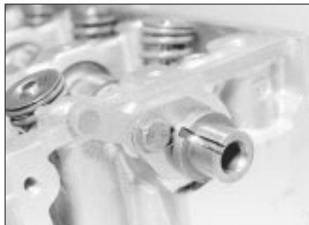
6.7 Camshaft retaining thrust plate
