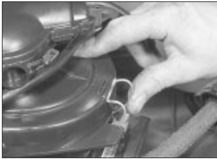
2.7a Release the spring clips . . .
