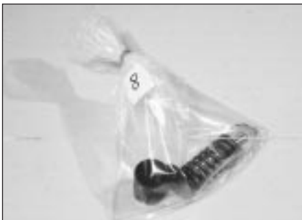
6.7 Place each valve and its associated components in a labelled polythene bag
