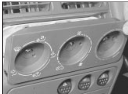
26.21 . . . Withdraw the heater control surround
