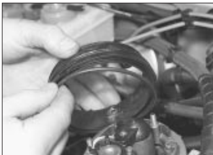
11.11b . . . and recover the O-ring
