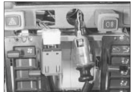
4.7 Heated rear window switch and cigar lighter removed from facia
