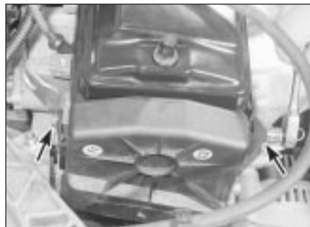
6.1a Undo the two retaining bolts (arrowed) . . .
