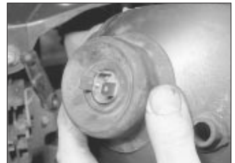
8.6 . . . remove the rubber cover . . .
