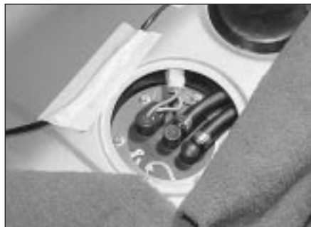
5.3 Fuel pump locations and connections
