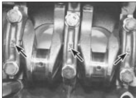
8.14 Main bearing cap identification markings (arrowed)
