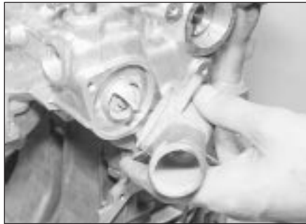
4.4 Removing the thermostat housing cover on XV, XW and XY series engines
