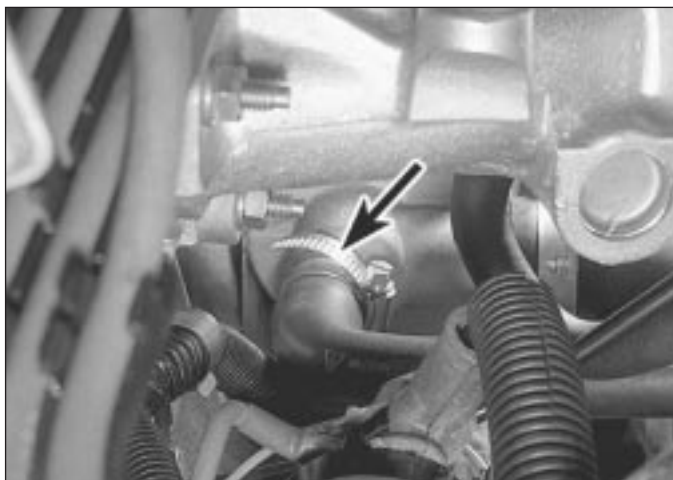
8.17a On TU series aluminium block engines, disconnect the hoses (arrowed) from the coolant pump housing
