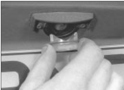
8.22 Remove the rear number plate light lens . . .
