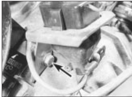
2.4a Air cleaner mounting bracket bolt (arrowed) . . .
