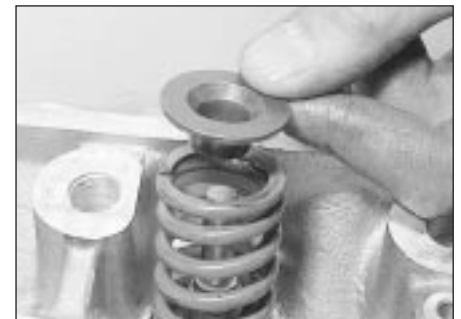
6.4b . . . Release the compressor and remove the spring retainer . . .
