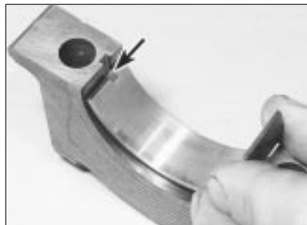
13.84 Ensure that the tab (arrowed) is correctly located in the cap when fitting the bearing shells
