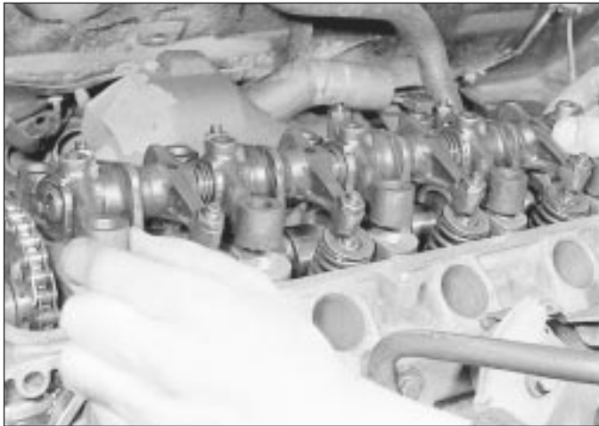
7.26 Removing the rocker shaft assembly
