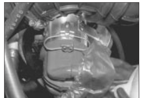
4.5 Pull back the plastic cover then unclip and remove the distributor cap
