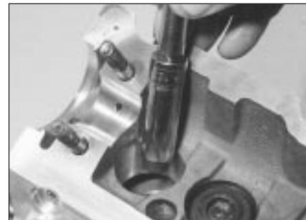
6.28 Fitting a valve stem oil seal using a socket
