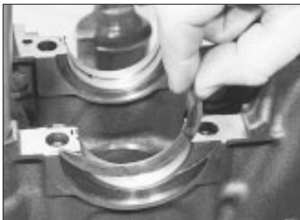
13.83 Fitting a thrustwasher to No 2 main bearing upper location - TU series cast iron block engines
