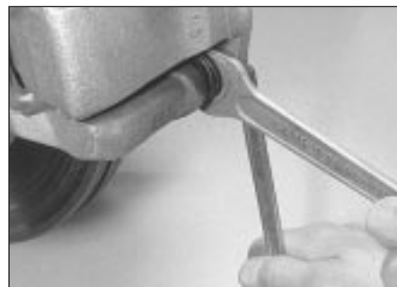
4.19 Unscrewing the lower caliper guide pin bolt (1.9 GTI)
