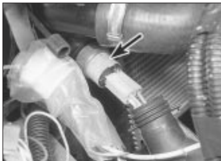
5.4a Disconnect the thermo-switch (arrowed) . . .
