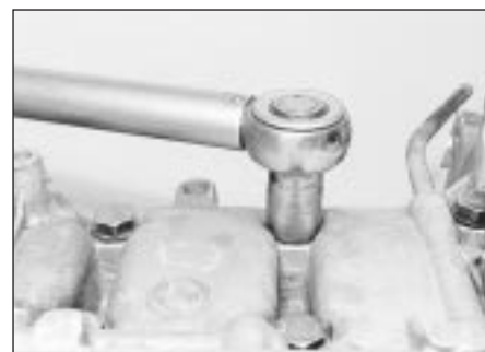
13.45 Tightening the main bearing/casing bolts
