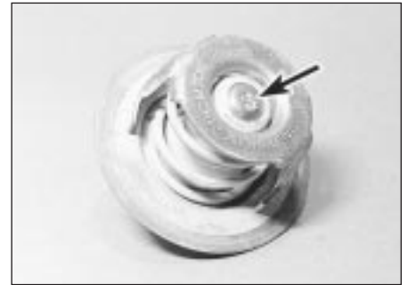
4.9 Thermostat temperature rating (arrowed) stamped on base
