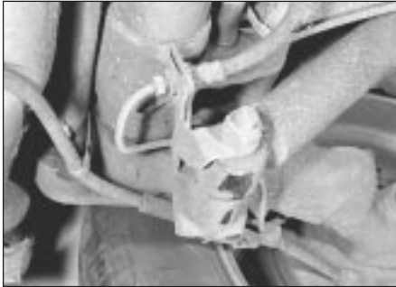
10.2 Rear shock absorber bottom mounting
