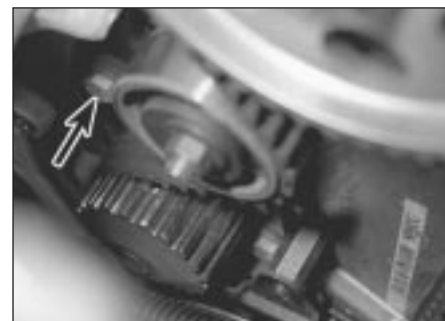
8.23 Coolant pump securing bolt (arrowed) on TU series cast iron block engines
