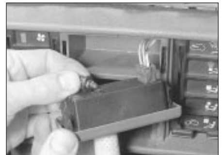
9.11 Removing digital clock illumination light bulb
