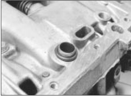
3.45 Locate a new O-ring oil seal on the transmission casing
