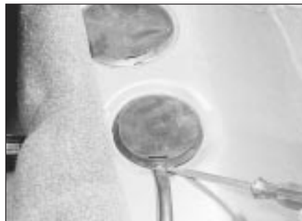
6.3a Remove the circular plastic covers . . .
