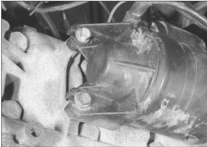
9.5 Starter motor brush end bracket retaining bolts on XV, XW and XY series engines
