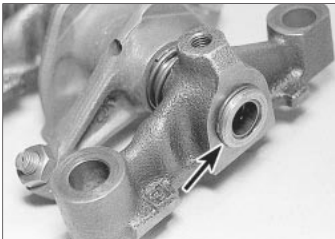
6.4a Prise off the circlip (arrowed) from the end of the rocker shaft . . .
