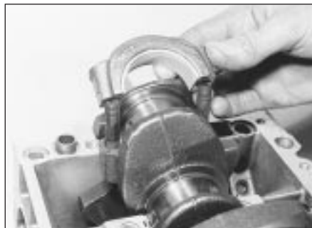
7.5 Remove the big-end bearing caps
