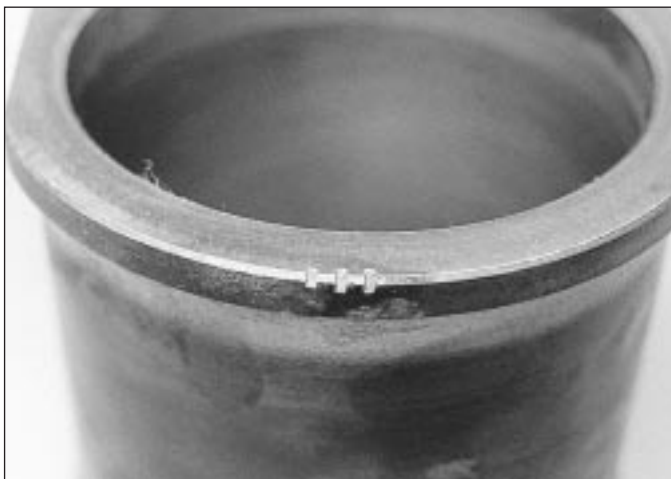
9.18 Cylinder liner size group marking
