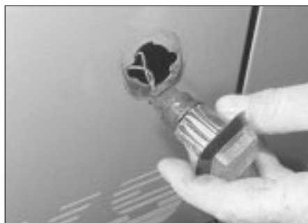
8.12 Removing the front direction indicator side repeater on later models
