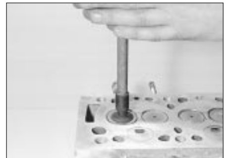
6.21 Grinding-in a valve
