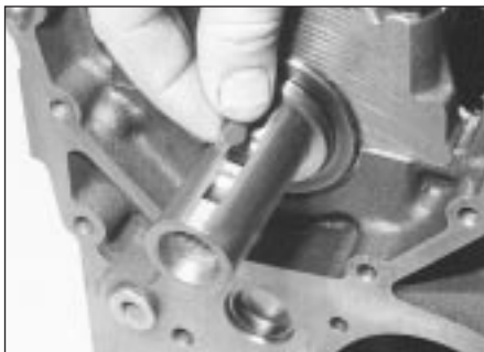
8.12b . . . and remove the Woodruff key
