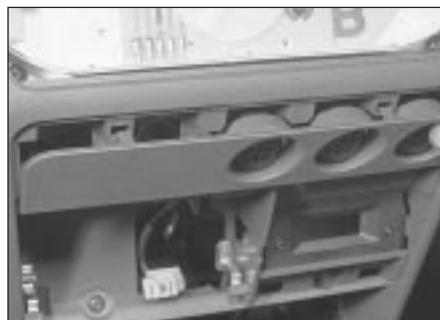
4.13c . . . and withdraw the switch panel surround
