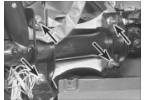
26.29 Steering column mounting nuts (arrowed)
