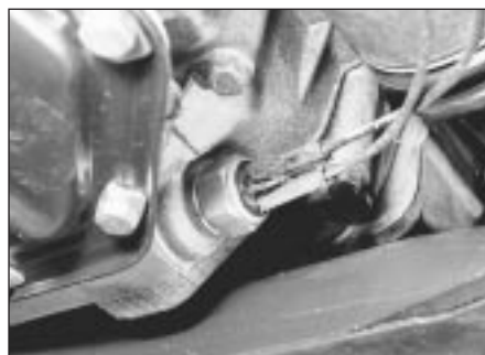
4.18 Reversing light switch location on the BH3 transmission
