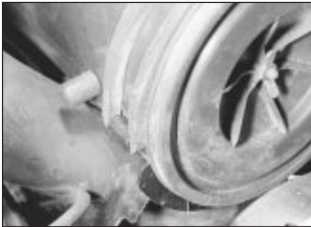
2.2 On all engines except TU series, release the air cleaner rubber straps from the mounting brackets
