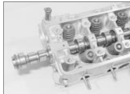
6.8 Removing the camshaft
