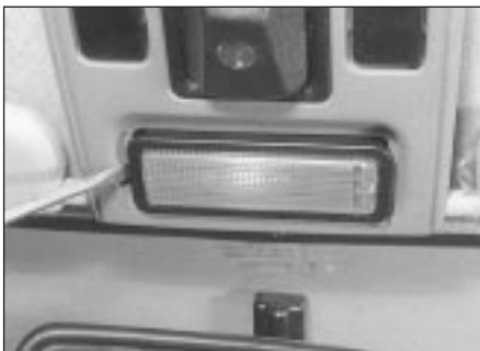
9.3 Prise out the interior light for access to the bulb
