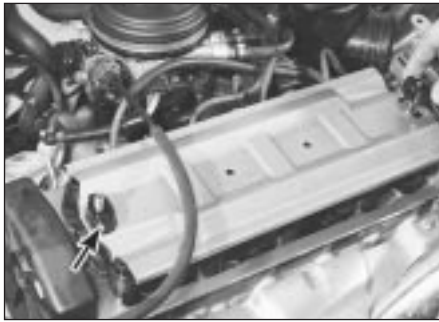
4.6a Lift off the spacers (second one arrowed) . . .
