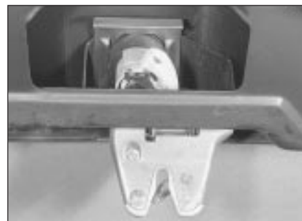
17.3 Tailgate lock and lock barrel
