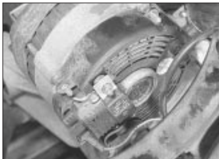
6.4 Alternator wiring connections
