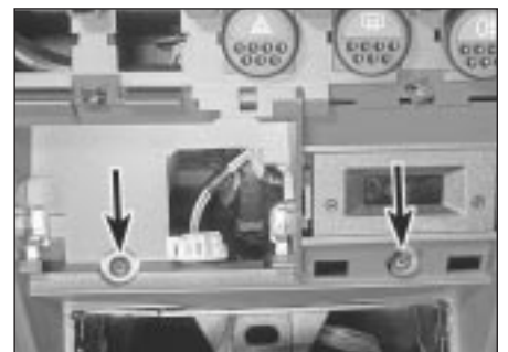
26.36 Front fascia panel screws (arrowed)
