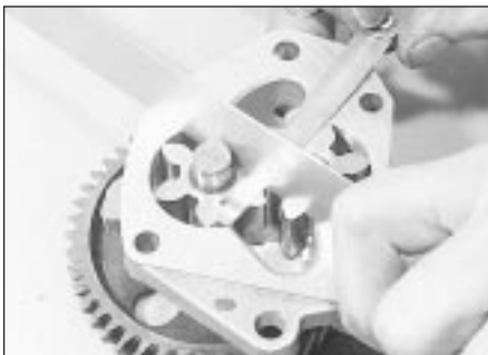
5.5 Checking oil pump gear endfloat
